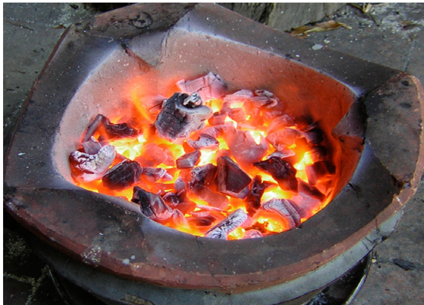
Figure 9. Jiko Kisasa SOURCE: Field photos
